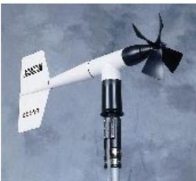
For offshore and marine use, **Model 05106, Wind Monitor-MA** features special waterproof bearing lubricant and a sealed, heavy duty cable pigtail in place of the standard junction box. Separate signal conditioning for voltage or current outputs is available.
